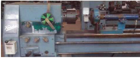
Fig. 2: Friction welding setup
