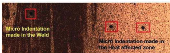
Fig. 12 Indentations made on the fw joint during Vickers hardness test
