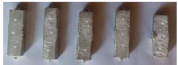
Fig. 5. Samples from FW joints subjected to hardness test
